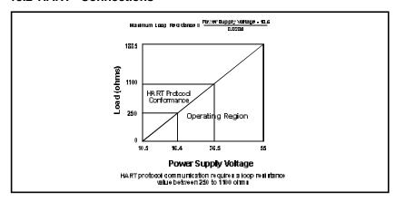
Maximum resistance versus DC loop voltage
